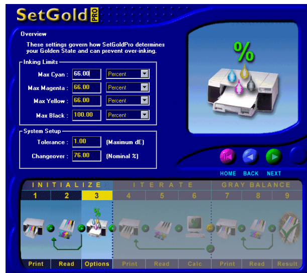
Figure 4.7 The Inking Limits screen
