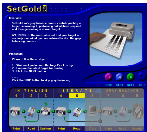
Figure 4.10 The Read Gray Balance target screen
