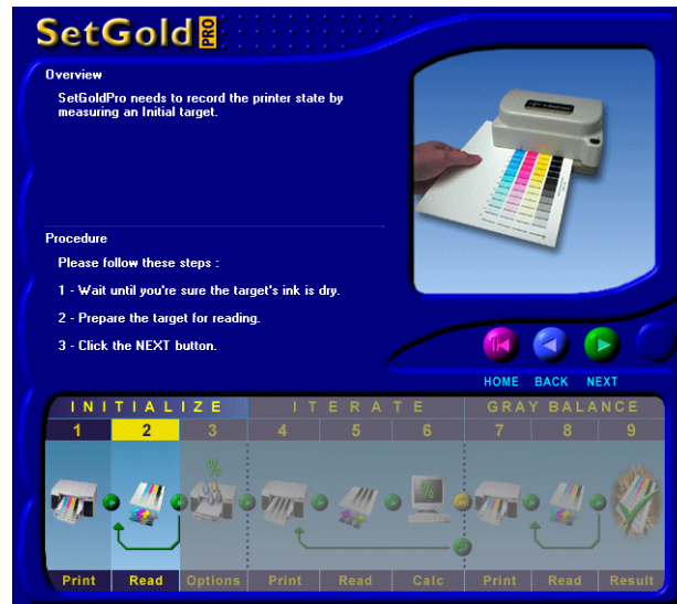
Figure 4.5 The Read Initial target screen
