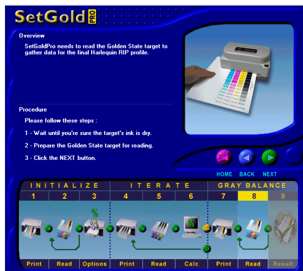
Figure 4.14 The Read the Golden State target screen
