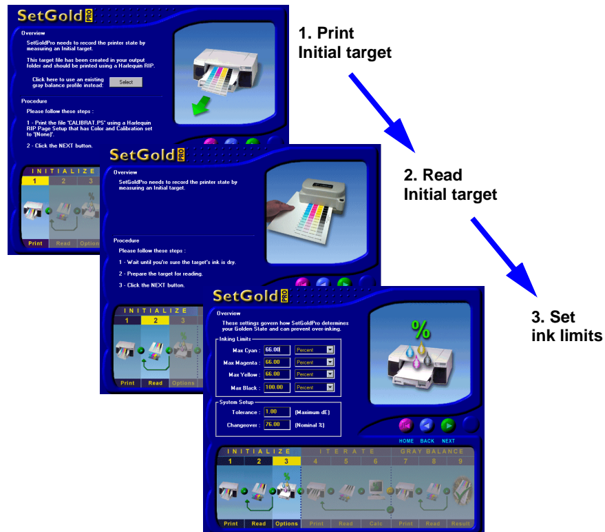
Figure 4.2 The Initialization process
